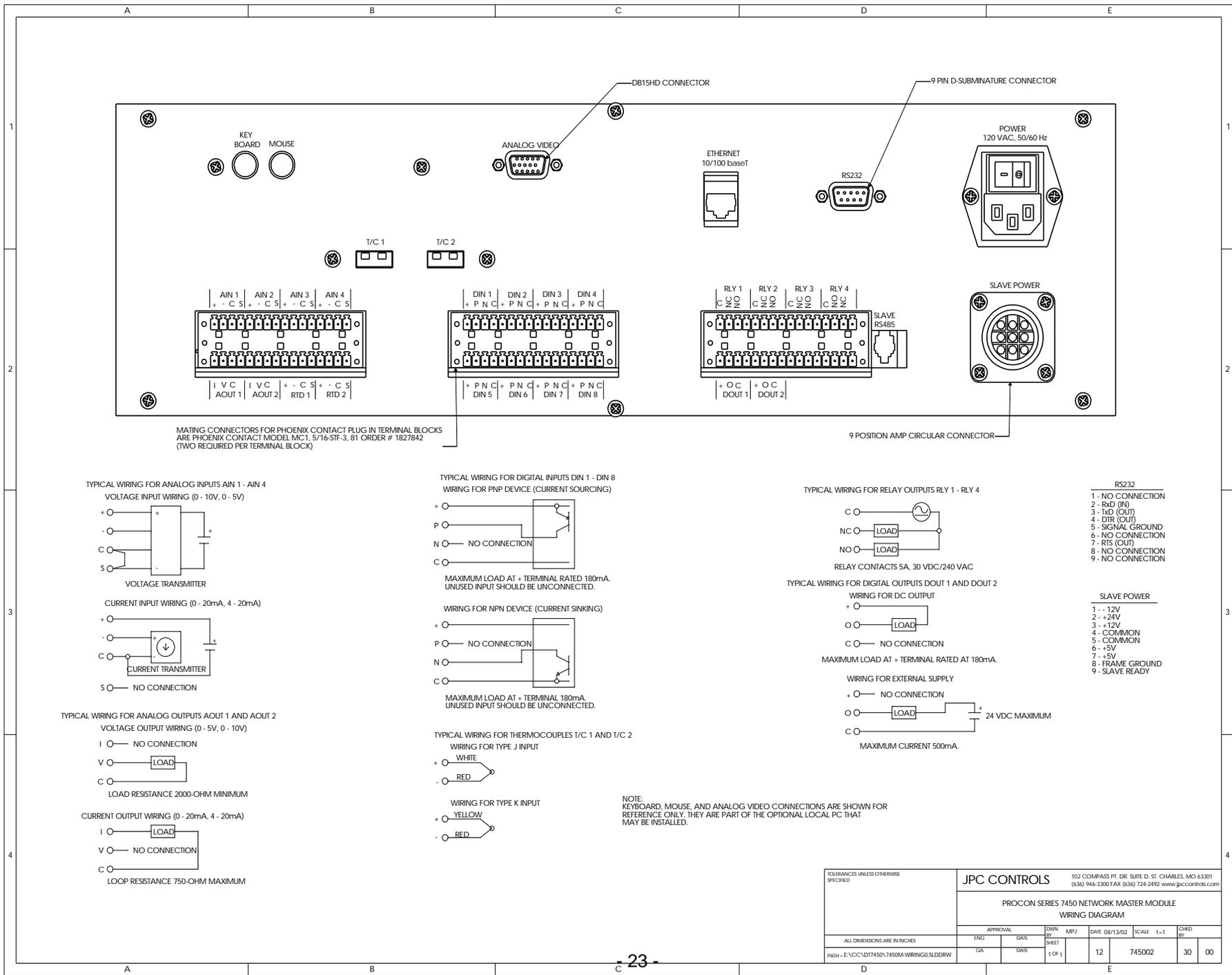
MATING CONNECTORS FOR PHOENIX CONTACT PLUG IN TERMINAL BLOCKS ARE PHOENIX CONTACT MODEL MC1, 5/16-SIF-3, 81 ORDER # 1827842 (TWO REQUIRED PER TERMINAL BLOCK)
