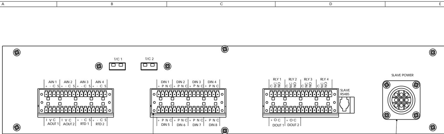
MATING CONNECTORS FOR PHOENIX CONTACT PLUG IN TERMINAL BLOCKS ARE PHOENIX CONTACT MODEL MC1, 5/16-STF-3, 81 ORDER # 1827842 (TWO REQUIRED PER TERMINAL BLOCK)
